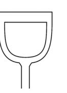
This is the least efficient and least ergonomic version. Newer versions of the T-shaped handles with more rounding show fewer problems, except for rescuers with small hands, where the entire handle is too big and does not allow a proper grip any more.
